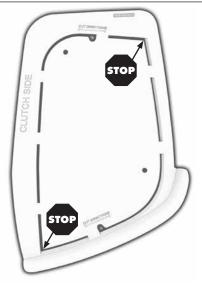
Its time to start cutting. We suggest a standard jigsaw or an air "body" saw. In all cases, you will **start at one of the "keyholes"** in the template, and **stop at the "hard corners"** as shown. Make sure to cut through all the tabs in the template. We suggest starting at the keyhole closest to the middle of the lid first. Once the template is free from the lid, it can be discarded. You will now see the line you scribed in case you need to do any trimming before proceeding.
