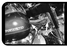
Stock Harness and Amplifier's Harnesses Passing From Fairing To Just In Front Of Tank (Arrow A). Cable Tying the Harnesses To The Main Bike Harness Just In Front Of The Tank (Arrow B) Allows The Amp Harnesses To Go Up Towards The Tank's Chrome Console Easier And Makes For a Cleaner Install.
