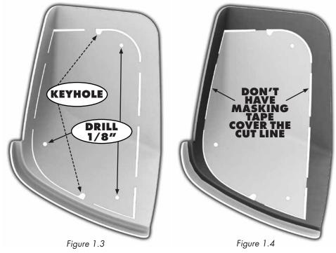
Underside of Template No Masking Tape Underside of Template With Masking Tape Applied Around Perimeter
